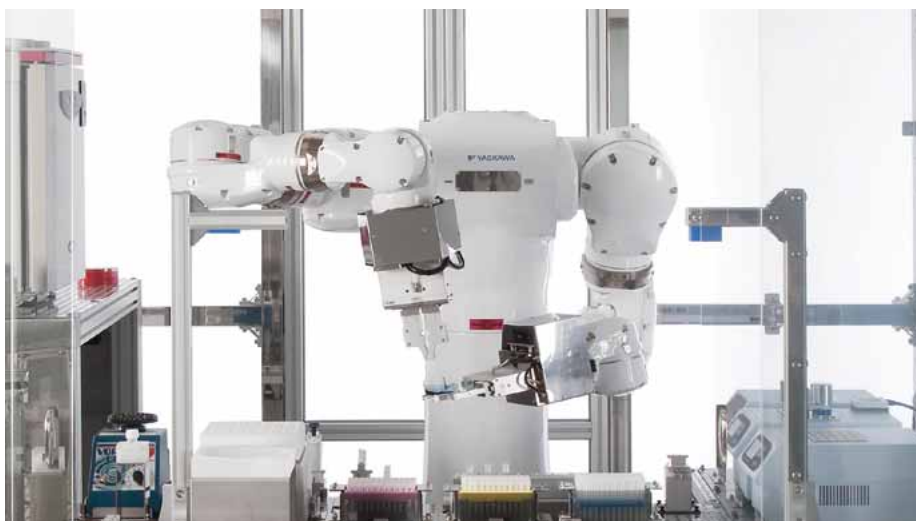
Abb. 3: The MOTOMAN dual arm robot in a biomedical cell where it performs all the necessary tasks in a laboratory environment.
